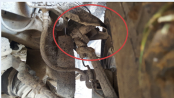
This upper suspension arm collapsed under the increased leverage being applied to it due to a ball joint spacer being fitted.
