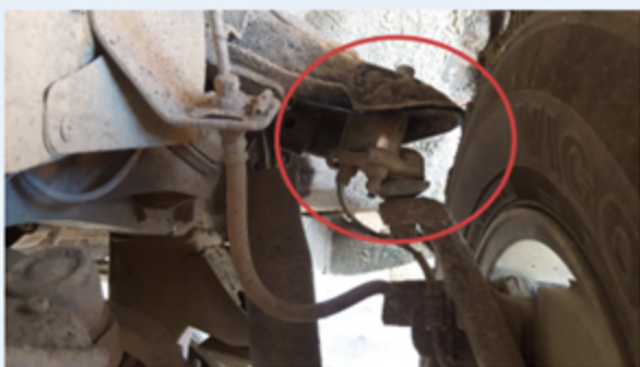
Ball joint spacers such as this increase the load on suspension arms, and as such are not suitable in all instances. LVV certification is required to confirm their suitability.
